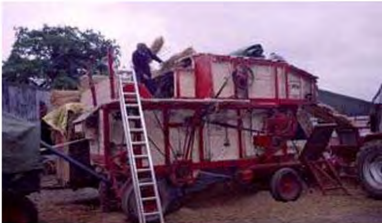
Figure 6 A threshing machine with a comber attachment for producing combed wheat (Devon)
